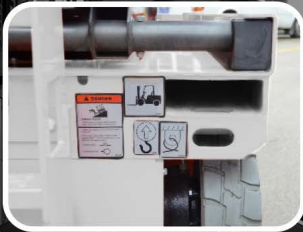
Standard transportation forklift holes and crane holes
